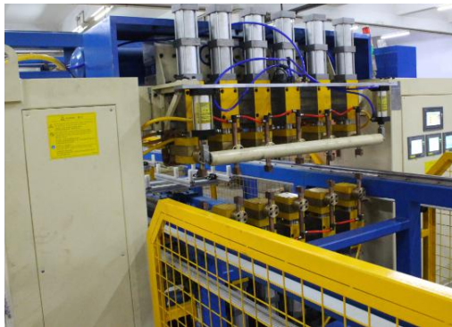
IBC吨桶框架网片龙门式自动焊接专机 IBC Tank Frame Automatic Welding Machine
